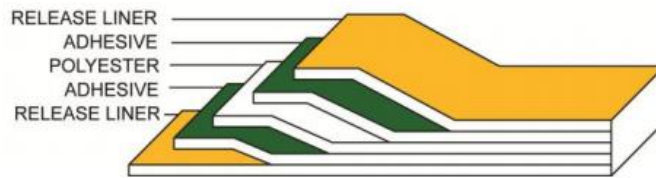
Figure 1 Anatomy of the heat seal adhesive tape [25]
