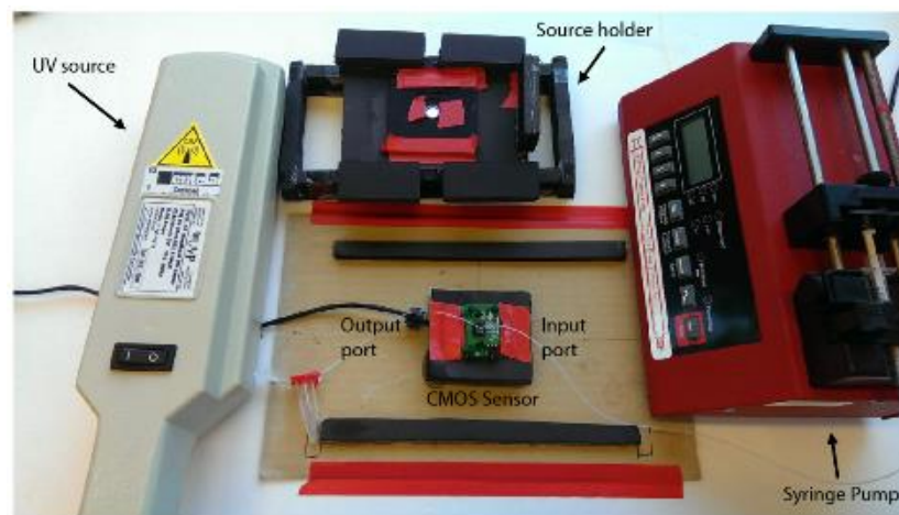
Figure 16 Imaging set up to perform lensless imaging [46]
