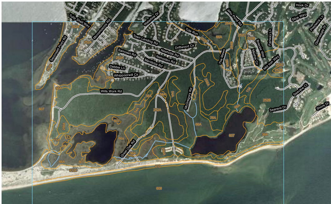
Figure 10.4. Soil survey data for the site shown in the previous figure (10.3). Tidal marshes are represented by map units 66A (Ipswich, Pawcatuck, and Matunuck peats) and 54A (Freetown and Swansea mucks), while units 610 are beaches. (USDA Natural Resources Conservation Service)
