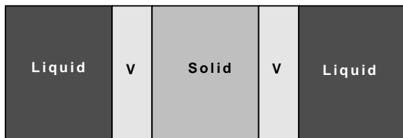
FIG. 1: Conceptual representation of the experiment showing the sandwich-like geometry with three chambers, each pair of which is separated by a region of liquid helium-filled porous Vycor glass, V. In operation a temperature difference is applied across each of the regions of Vycor, which keeps the liquid reservoirs from freezing.
