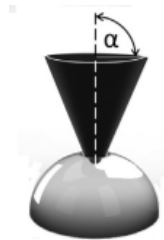
Figure 17: Sneddon's model with conical indenter[30]
