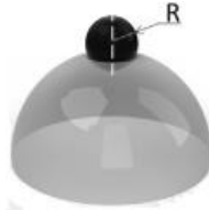
Figure 16: Hertzian mechanics model with a spherical indenter of radius R [30]
