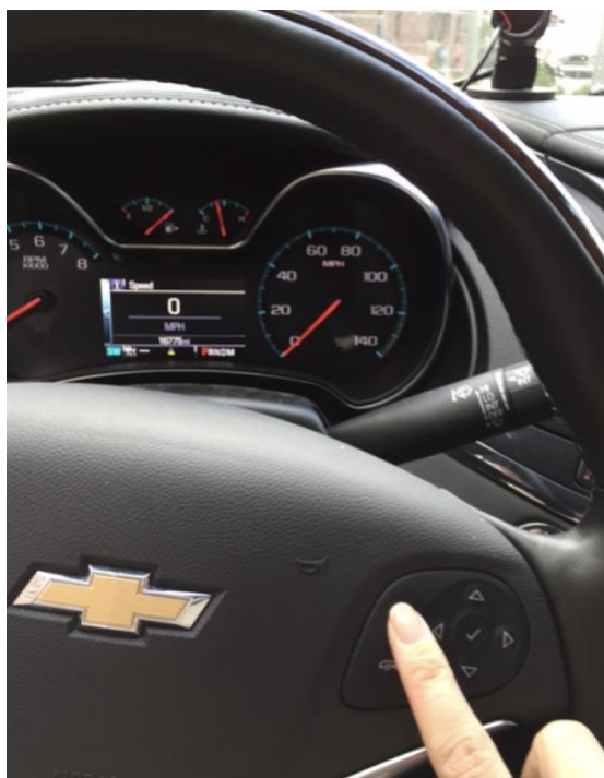
Figure 9. Additional small display in the instrument cluster, 2014 Chevrolet Impala
