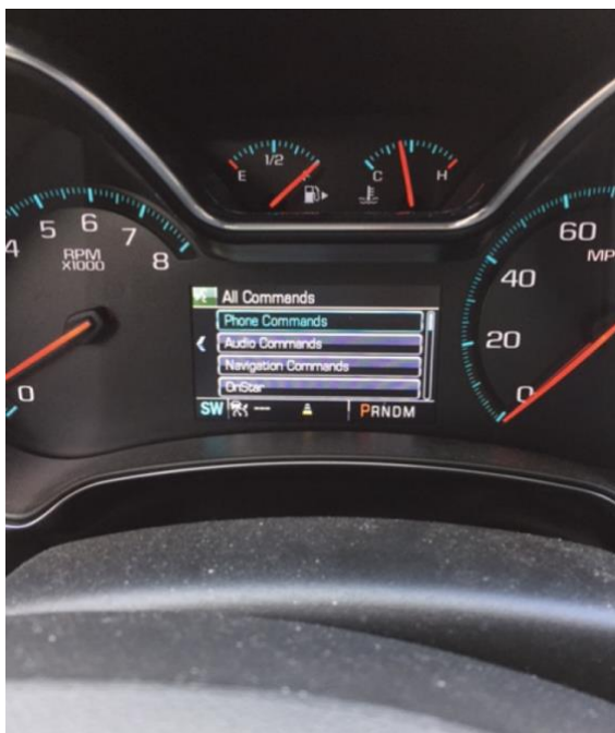
Figure 9. Additional small display in the instrument cluster, 2014 Chevrolet Impala
