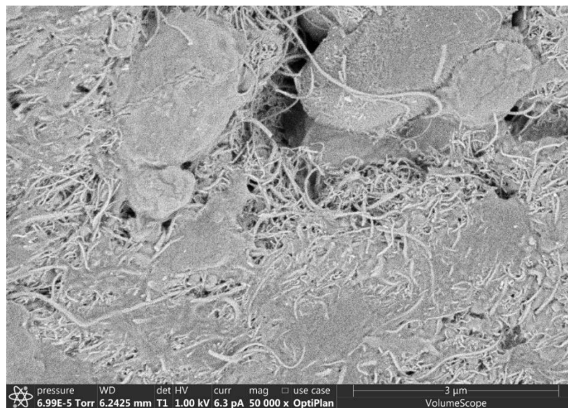
Figure 14: Scanning Electron Microscopy image of the surface of CNT-HDPE composite powder. The CNTs are visible as threads that are pressed into the HDPE powder surface
