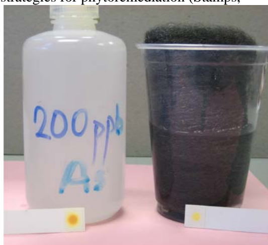
Figure 2. Arsenic removal from contaminated water by steel wool
