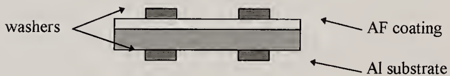
Figure 4.2: AF 1601 holography sample preparation
