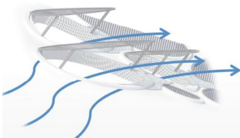
Figure 45: Operable Panels for Passive Ventilation
