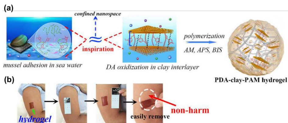
Figure 3. (a) Schematic of hydrogel formed by polymer intercalating into nanoclay sheets with polydopamine. (b) Photographs of hydrogel that sticks to human skin and can be easily removed (reproduced from [37], copyright 2017 ACS).
