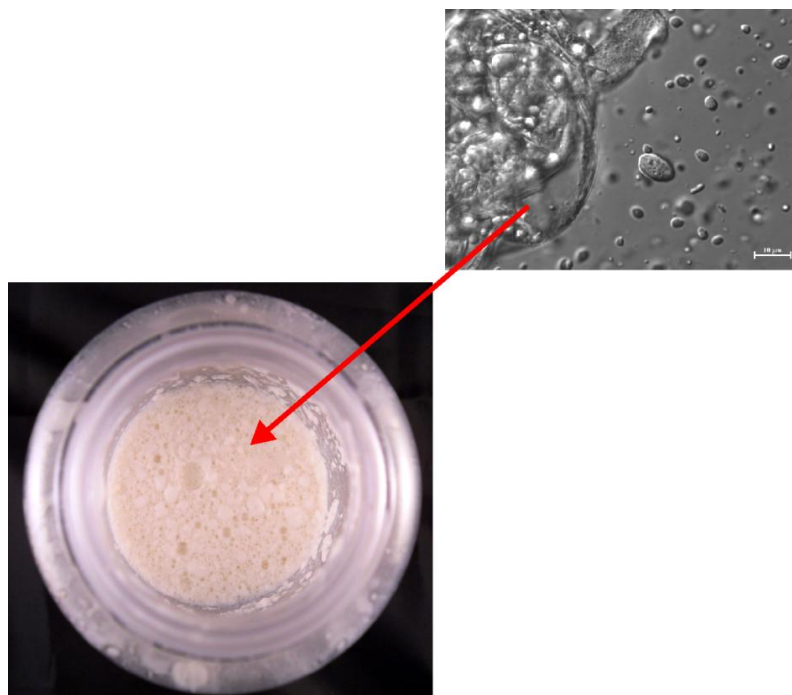
Figure 7.4: Photograph and micrograph of filled hydrogel particles formed from 30% (vol/vol) lower phase and emulsion and 70% (vol/vol) upper phase after centrifugation at 1,000 g for ten minutes. Note coagulated protein on surface of mixture, and coagulated protein (left) and free particles (right) in micrograph
