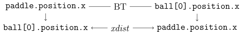
Figure 5.7: The data dependence graph for the x distance between ball and paddle. The input is a value for the x distance ( xdist ). We randomly select which of the ball or paddle x positions to set first. The other x position is then computed from the input distance and the position of the variable that was set first.
