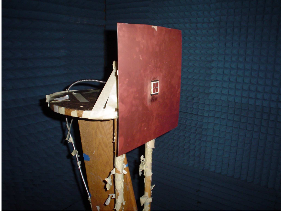
Figure 93 – Patch with four 9mm long, 1mm wide slots mounted on AUT positioner in the far field range. The ground plane is 12×12”.
