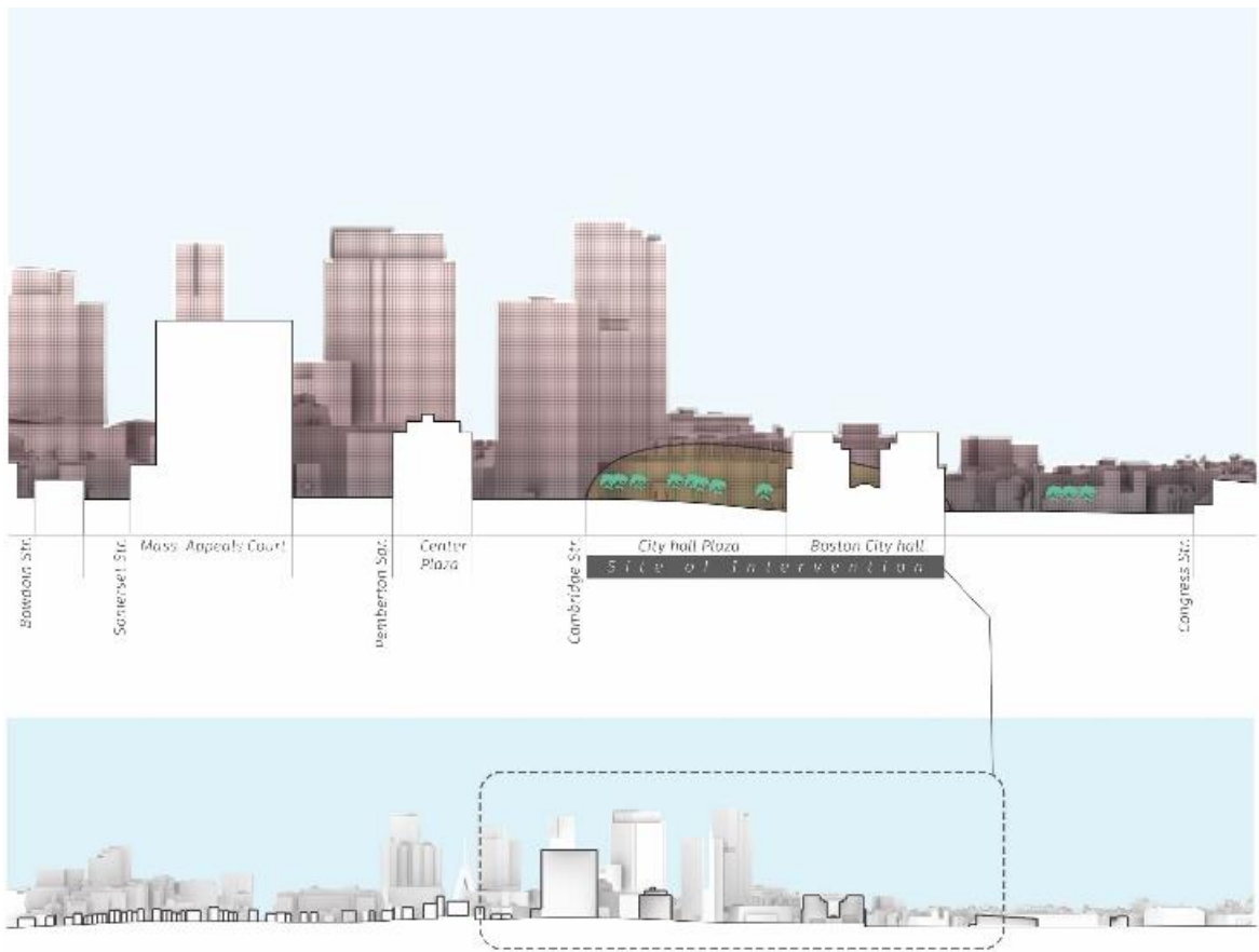
Figure 10: Section through the site depicting Congress Street and Cambridge Street, and a contour difference of 13 feet. Image by Author
