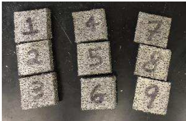
Figure 1.12: Samples of HS steel foam pre-impact testing
