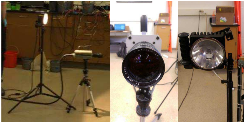
Figure 1.13: 4,500 fps high-speed camera and lighting
