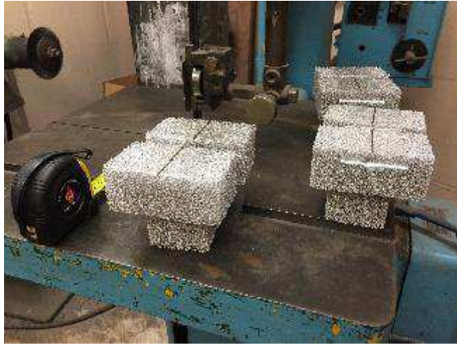
Figure 1.9: Pre-cut samples of aluminum foam
