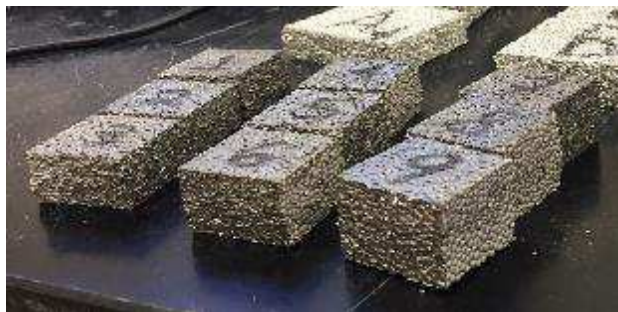
Figure 1.14: Samples of HS steel foam post-impact testing acquired, twelve samples were cut and the best nine of those were used in the tests. These nine optimal samples correspond to the visual geometry that they exhibit, such as straight
