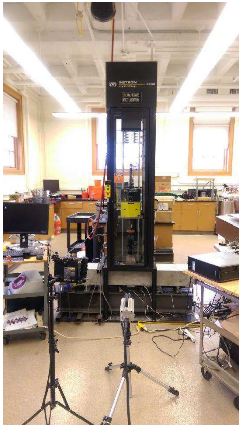
Figure 1.10: Instron dynatup 8250 impact testing machine and set-up
