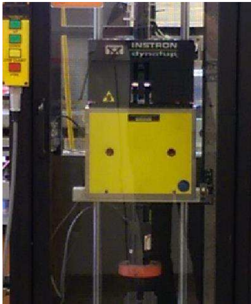
Figure 1.11: Impactor with mass
