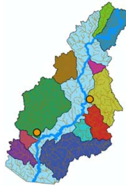
Figure 8: Hydrology model calibration points (indicated by gold circles). The two calibration points, Upper Ammonoosuc (upper right point) and the Passumpsic (lower left point) are each at the mouth of their respective rivers.
