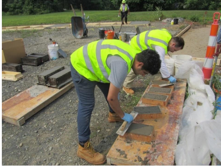
Figure 4.4: Placement of 6 in. x 12 in. x 3in. scaling test specimens
