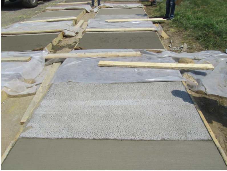
Figure 5.10 Panel group 5H is covered in a moist cover and 1I is uncovered with no curing methods
