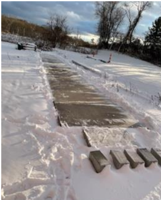
(a) Panels A, B, and C treated with NaCl after removal of snow on January 30 th , 2022.
