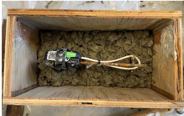
Figure 4.18 Thermal sensor in mold before concrete pour
