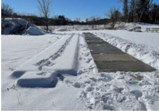
(a) Removal of snow on panels D, E, and F which are subjected to MgCl_2 (Right). Panels G, H, and I treated with blended brine on accumulated snow (Left) on February 26 th , 2022.
