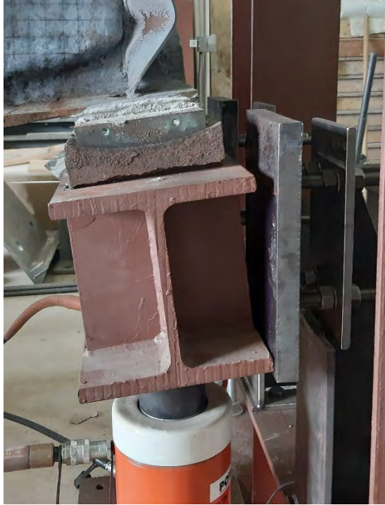
Figure 6.7: Both experiments terminated due to inclination of load spread beam, located between hydraulic jacks and bridge bearing
