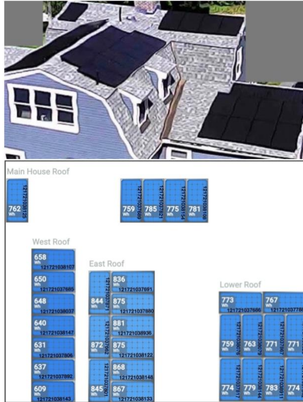
Figure 1: A residential solar array (top), and real-time panel-level generation
