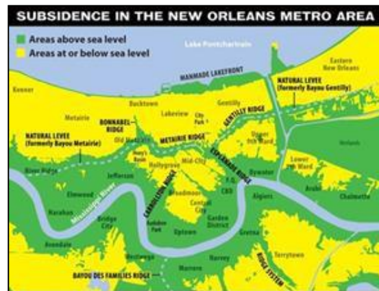
Figure 1: Subsidence in the New Orleans Metro Area. Source: Richard Campanella, 2018
